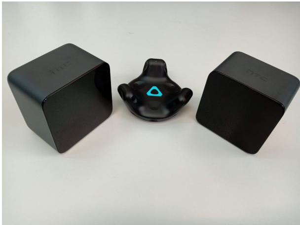
Fig. 5. HTC VIVE Base Stations (left and right) and Tracker (center).
