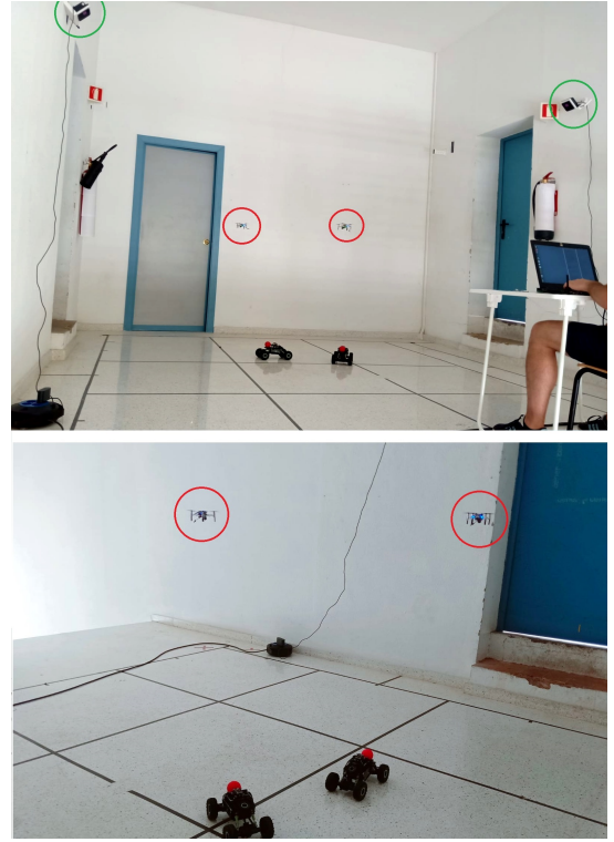
Fig. 6. Pictures of the testbed set-up for the multi-drone target tracking experiments. The Crazyflies are marked with red circles, and the lighthouse base stations, in green.
