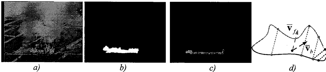
Figure 4. a) visual image of a fire. b) segmented fire. c) pixels belonging to the fire base. d) scheme of the final characterization: blue, pixels of the backward fire front, green, pixels of the forward fire front, red, pixels of the top of the flame.
