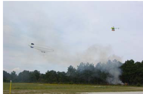
Fig. 1 An autonomous airship and a helicopter monitoring a fire in the COMETS experiments carried out in Louisa (Portugal).
