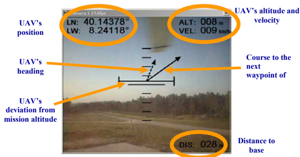
Figure 10. Teleoperation video camera with overlaid information.
