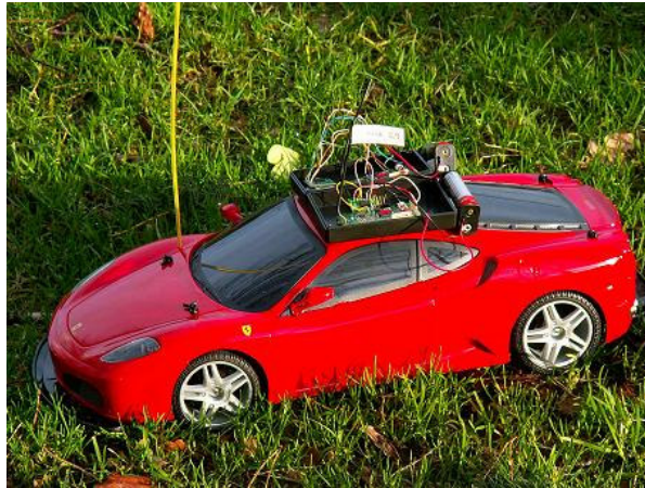
Figure 3 - Two sensor nodes with accelerometers attached to a wirelessly controlled toy car
