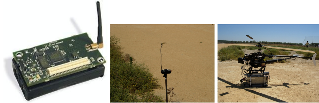
Figure 9.1: Left: Crossbow Node. Middle: a node with a dragonfly on the antenna for scale comparison. Right: helicopter carrying a node.
