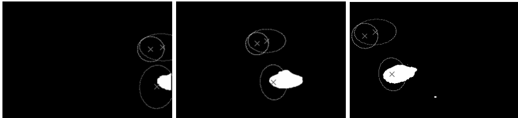
Figure 8.17: Heliv receives the information of the alarms from Marvin and updates its belief by using its infrared camera. This figure shows the estimated position and uncertainty of the alarms detected by Marvin projected on the Heliv's infrared camera.
