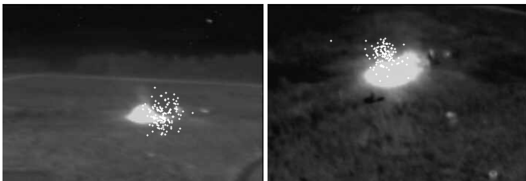
Figure 5.14: Fire detection experiment 1. Particles projected onto two images gathered by the two UAVs. The different points of view allow reducing the uncertainties.
