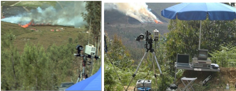
Figure 6.19: Two pictures of the actual deployment of the system. Only the frontal cameras are shown. Cameras in other places are also deployed (transmitting their images to the central station).
