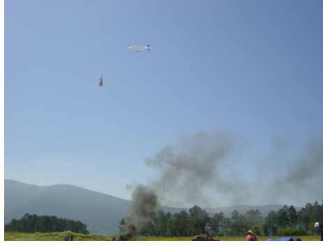
Figure 3.3: Two heterogeneous UAVs in a fire detection and localization mission. The important information is the location of the alarms. The UAVs should avoid generating false alarms.
