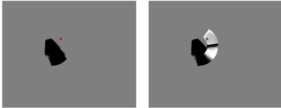
Figure 8.16: Marvin employs a grid representation to integrate the data gathered by its fire sensor. The red square indicates the actual position of the fire. High probability regions are extracted and approximated by Gaussian distributions. Due to false alarms, other high probability regions are also detected.
