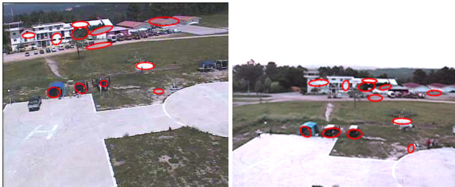
Figure 7.22: Blobs fulfilling the estimated homography between two images from different UAVs with video sensor and a digital photo camera, respectively.
