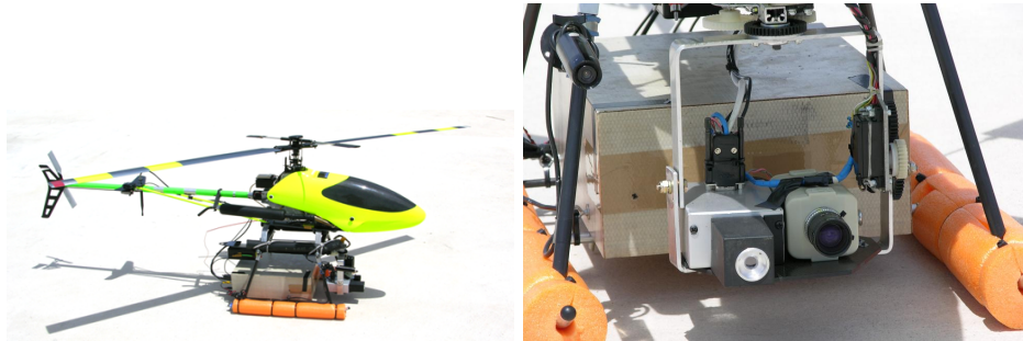
Figure 8.9: The Heliv teleoperated helicopter and its electronic box (the pan and tilt unit can be distinguished).
