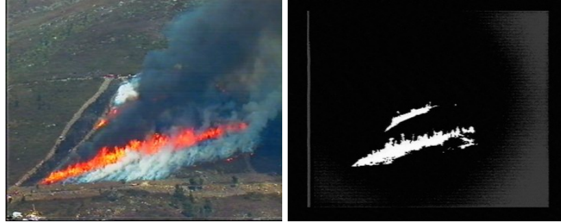
Figure 6.8: A visual (left) and an infrared (right) images of the same fire at approximately the same time instant. Infrared images are not affected by smoke, and therefore they also provided negative information. On the other hand, although the fire front can be occluded by smoke in visual images, they provide accurate measurements of the height of the flames.
